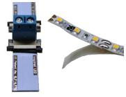
A Matching (+) polarity of LEDs, insert flex strips into gaps between black sliding latches and beige bridge piece.
