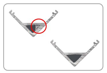
**Step 3:** Use razor blade and steel wool to remove any barbs or metal frays from the ends of the channel, as these will prevent end caps from being secured in step 11.
