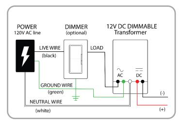
corresponding Hardwire System: Follow product instructions to connect to dimmable wall-switch and hardwire transformers.
