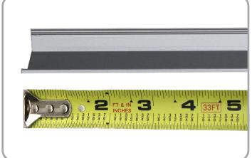
Step 2: Cut corner channel to length using sharp diamond blade saw.
