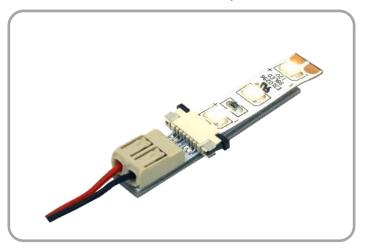
**Step 8:** Use compatible power source to test functionality. If lights do not turn on, double check polarities are properly matched. Repeat steps 4-8 to add connector to opposite side of flex.
