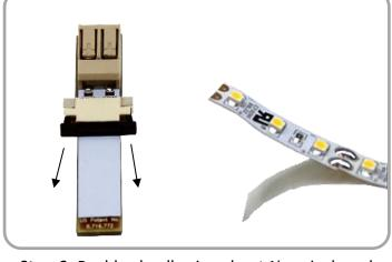
**Step 6:** Peel back adhesive about ½ an inch and pull open black latch on Micro-Lock. Insert LED flex between black latch and beige bridge connector, then slide latch firmly closed.
