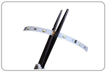
**Step 5:** If using pre-cut LED strips with direct-solder leads, skip to step 9. If modifying, use scissors to cut LEDs to length along copper pads.
