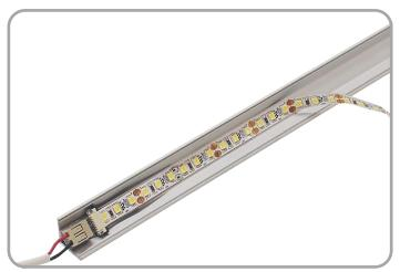
**Step 9:** Remove adhesive backing from LED strip and connectors. Carefully align with end of aluminum channel and adhere strip along the center.
