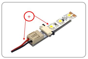
**Step 7:** Identify the polarity as marked along the strip to determine polarity of wiring. Strip back wire about ¼ inch and insert into Micro-Lock. (*Positive wire aligns with (+) side of LED flex strip.*)
