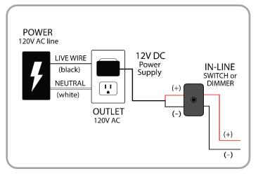
**Plug-in System:** Follow corresponding product in-line instructions to connect panels to accessories and plug-in power supplies.
